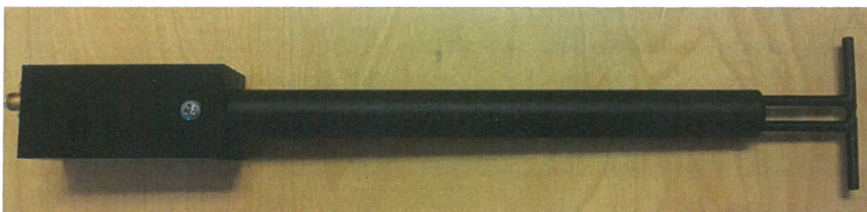
Figure 1 – MVG COMOSAR Validation Dipole
