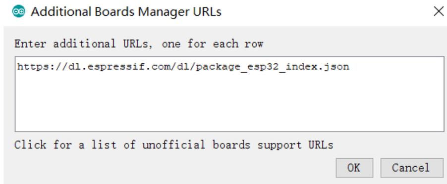
Also, in the "Preferences" setting page, you can set some display parameters, such as the editor text size, adding line number display, compiling/burning log prompts, and other auxiliary content. After saving the settings, select the "Tools" tab, point the mouse to the "Development Board" option, find the "Development Board Manager" in its sub-directory, and click Open.
