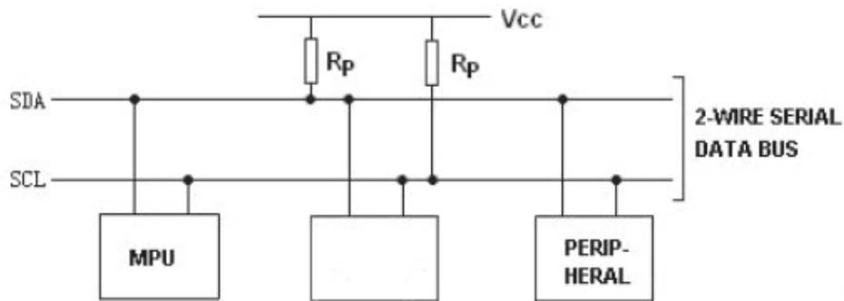
**Figure 7. Typical I<sup>2</sup>C-Bus Configuration**
