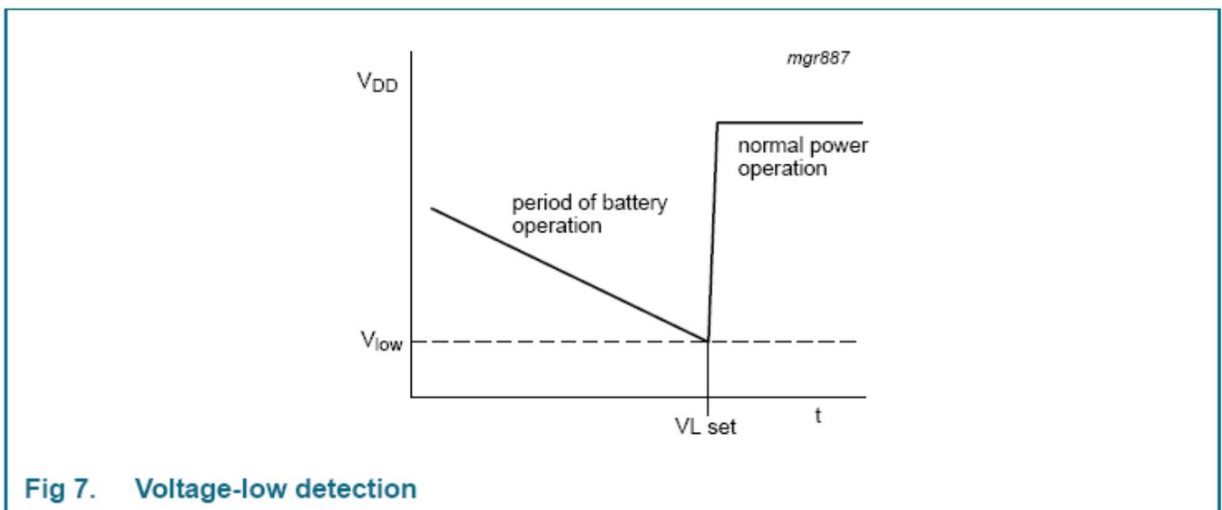
**Fig 7. Voltage-low detection**
