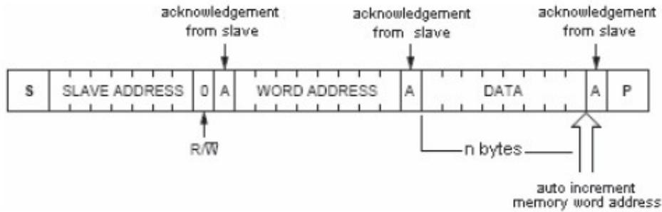
**Figure 11. Master transmit to slave receiver(write mode)**
