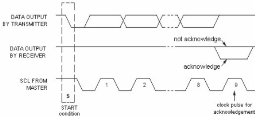
**Figure 10. Acknowledgement on the I2C bus**
