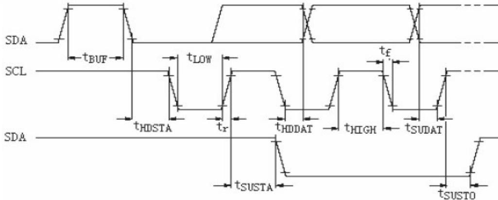
**Figure 1: I<sup>2</sup>C-bus timing waveform**
