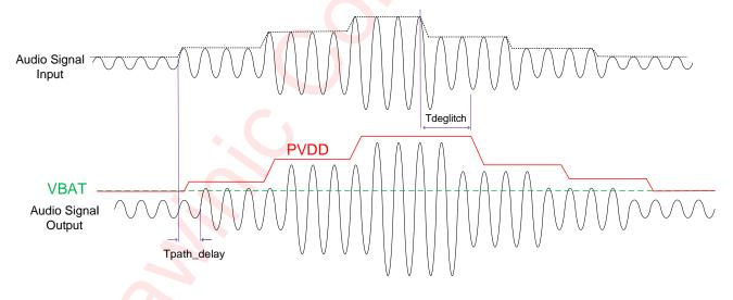
Figure 14 Boost Circuit Behavior in Smart Boost 2 Mode
