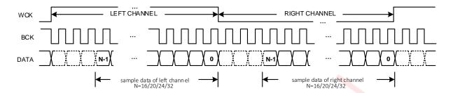
Figure 11 I<sup>2</sup>S Timing for Right-Justified Mode
