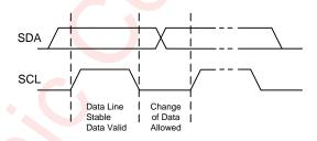
Figure 15 Data Validation Diagram
