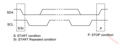
Figure 16 I<sup>2</sup>C Start/Stop Condition Timing
