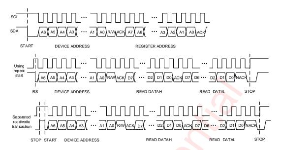
Figure 19 I<sup>2</sup>C Read Byte Cycle
