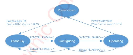
Figure 7 Device operating modes transition
