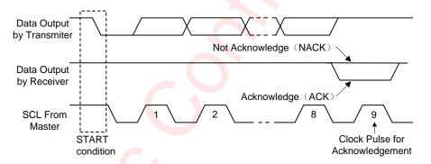
Figure 17 I<sup>2</sup>C ACK Timing
