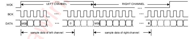
Figure 10 I<sup>2</sup>S Timing for Left-Justified Mode
