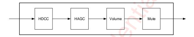
Figure 13 Block Diagram of DAP
