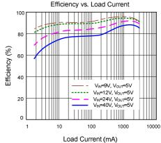
Figure 2. Efficiency vs. Load Current
