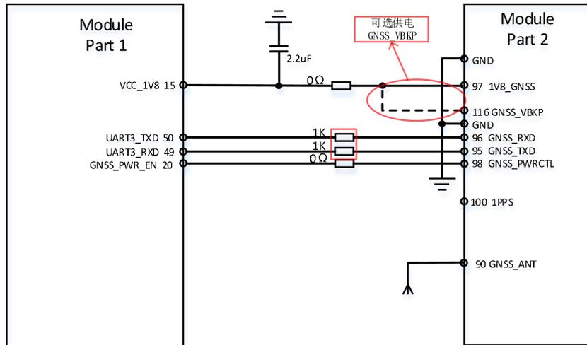
Figure 1: GNSS reference schematic diagram (non-independent GNSS solution)
