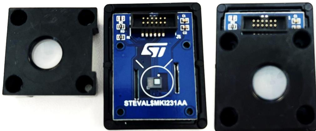
The lens holder can be 3D printed and the 3D drawing file for 3D printing can be downloaded at the following link: [3D lens holder for TMOS63-10](#)
